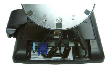
• Connect one end of the **serial touchscreen cable** to the rear side of computer and the other to the LCD monitor. Secure the cable under the cable management clip
